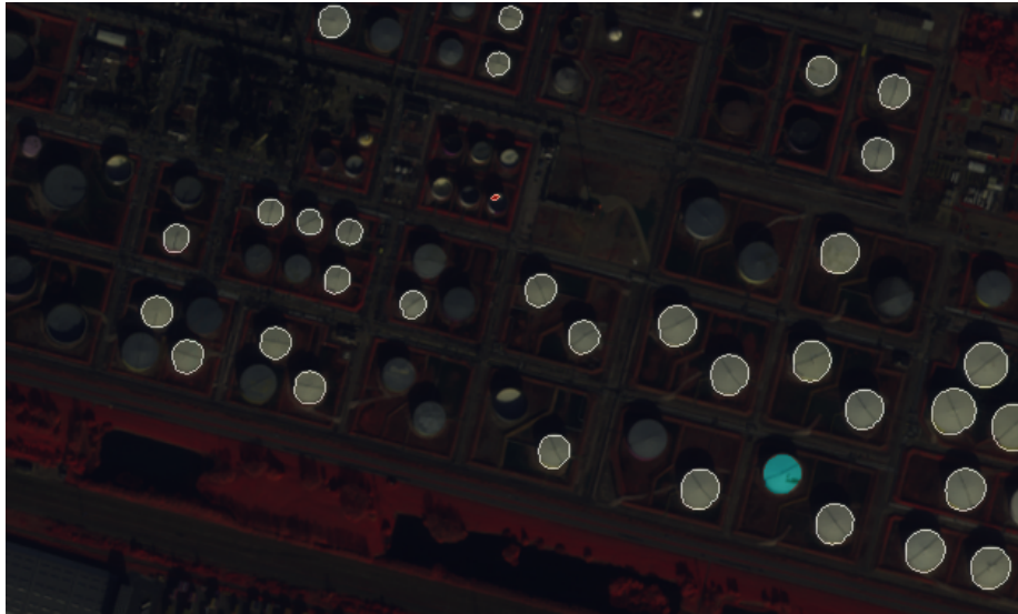
Figure 13: Petroleum tank extraction on Le Havre harbor QuickBird image(©Digitalglobe). Correct detections are surrounded by white boundary, false positive are given in red while false negative are given in cyan.
